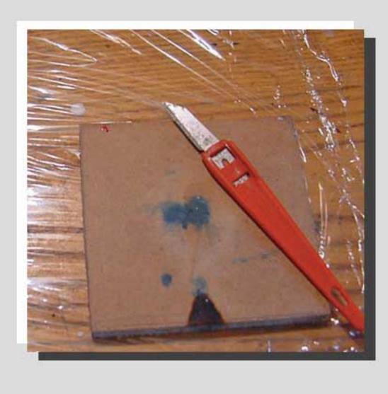
2. First cut a piece of MDF 50mm x 50mm square. Place masking tape around the edge of the MDF to create a reservoir to hold the plaster. Within the reservoir and on the base of the MDF place a square of the same size of Clingfilm. The purpose of this is to act as a barrier between the plaster and the MDF so that the two will easily separate.
