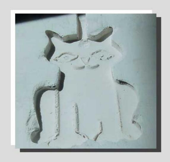
6. To release the template from the plaster cut a sprue hole from the top edge of the plaster mould down to the template. The template can, with care, be removed from the mould using a bradawl or similar tool. (The sprue is effectively a funnel to allow the liquid metal to run into the mould).
