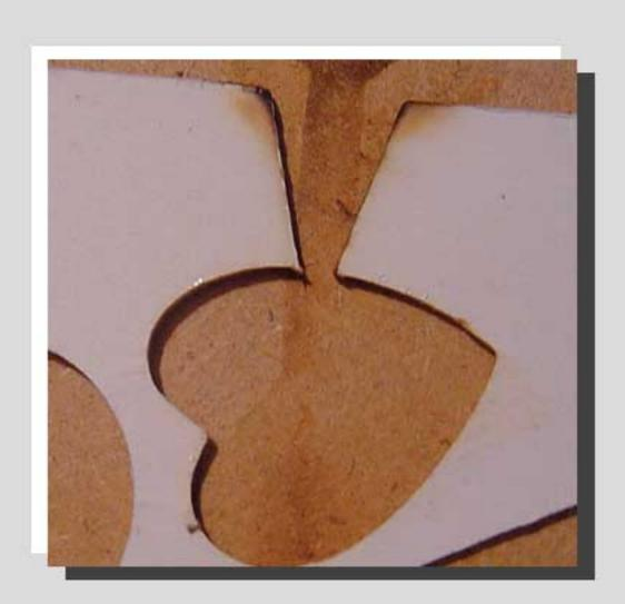
3. Using a second piece of MDF of the same size sandwich the card between the two pieces and place in the LT1 mould holder.
