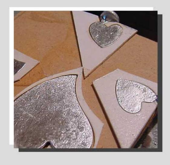
2. Select the negative heart shapes and place them individually or as a group on to a square of 50mm x 50mm MDF or similar material ensuring that each shape has a suitable sprue hole in line with the edge of the square. (The sprue is effectively a funnel to allow the liquid metal to run into the mould).
