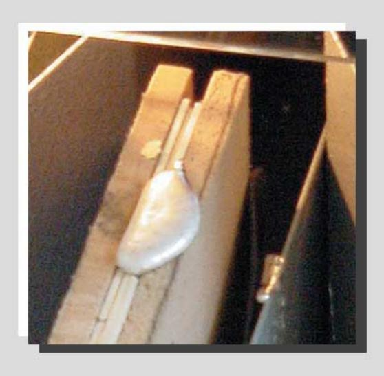
4. Moulds can be re-used as can be seen in the picture above. This mould was used 4 times and could still be used again. The pouring of metal was at high heat. More use could be made of a single mould at low heat but care should be taken that the liquid metal does not start to solidify.
