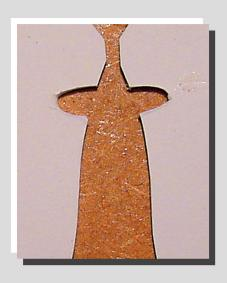
3. The finished card mould. The card mould is placed in between two pieces of 50mm x 50mm x 6 mm pieces of MDF.
