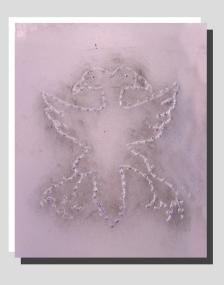
2. Carving out the design into one side of the cuttlefish to produce a mould. The cuttlefish is very soft and carves easily. Every mark is transferred to the cast so care must be taken in ensuring that the surface reflects the required pattern of the design.
