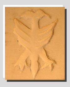
3. Adding sprue hole to mould. Angle Sprue hole of 8-10 mm to make a "pouring funnel" for the metal. No requirement for a vent as the cuttlefish bone is porous.
