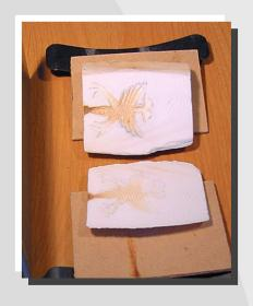
5. Flamefast LTI shuttle. The LT1shuttle with the cuttlefish mould clamped in position ready for insertion into the pouring channel of the LT1.
